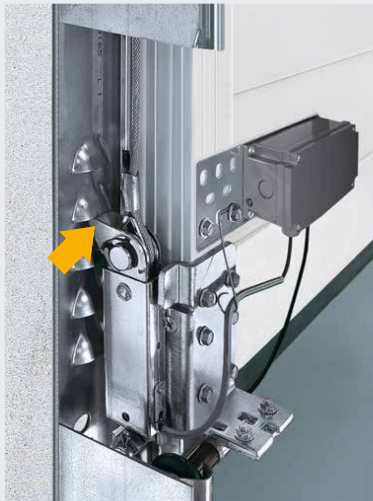
The locking hook of the anti-lift kit automatically latches if the door is forced upwards.
