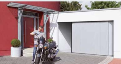
Hörmann's side sectional door opens to the side instead of upwards. This is particularly advantageous if, for example, the garage ceiling has to remain free to store items (such as ladders).
