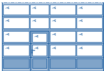
Sectional door ALR 67 Thermo with wicket door with trip-free threshold
